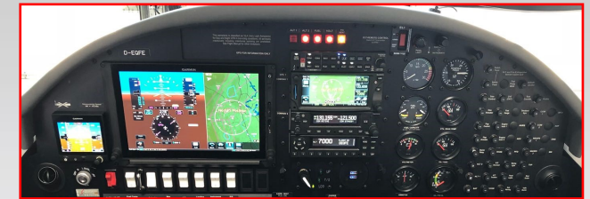
AQUILA A211G: Garmin G500 TXi glass cockpit and analog engine instruments
