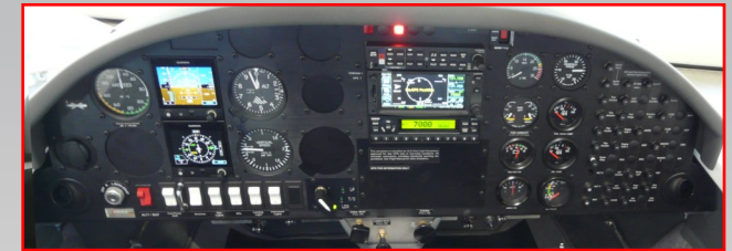
AQUILA A211: Analog flight and engine instruments
