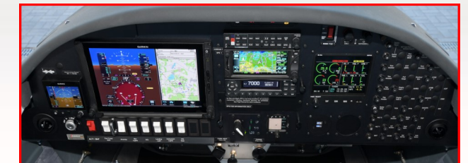
AQUILA A211GX: Garmin G500 TXi glass cockpit, Engine Monitoring System MVP 50P incl. Annunciator Panel
