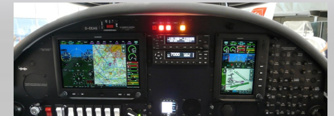
AQUILA A211G3X: 10" Garmin G3X Touch glass cockpit, 7" Garmin G3X Touch Digital Engine Monitoring System
