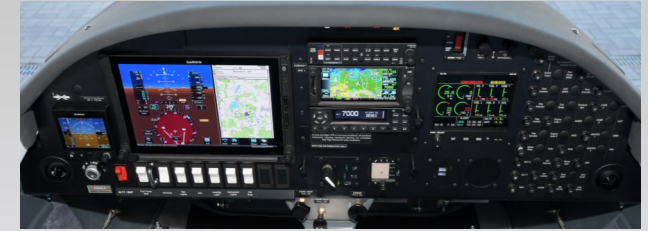
Garmin G500 TXi Glass Cockpit, Engine Monitoring System MVP 50P incl. Annunciator Panel
