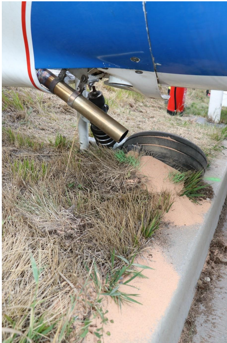
Figure 12: A small amount of fuel leaked from a fuel drain valve at the scene
