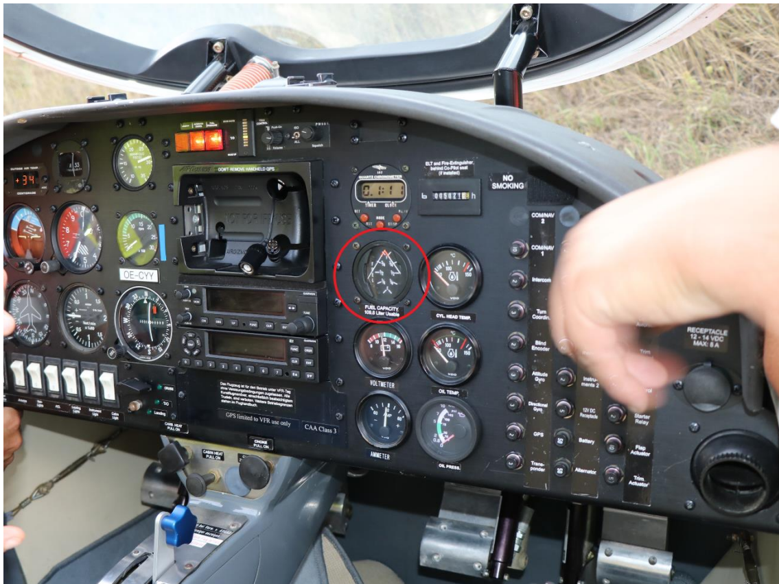
Figure 11: Position of fuel instrument indicators at the scene
