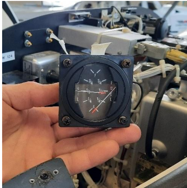
Figure 16: Indicators of the instrument when the GND contact is connected
