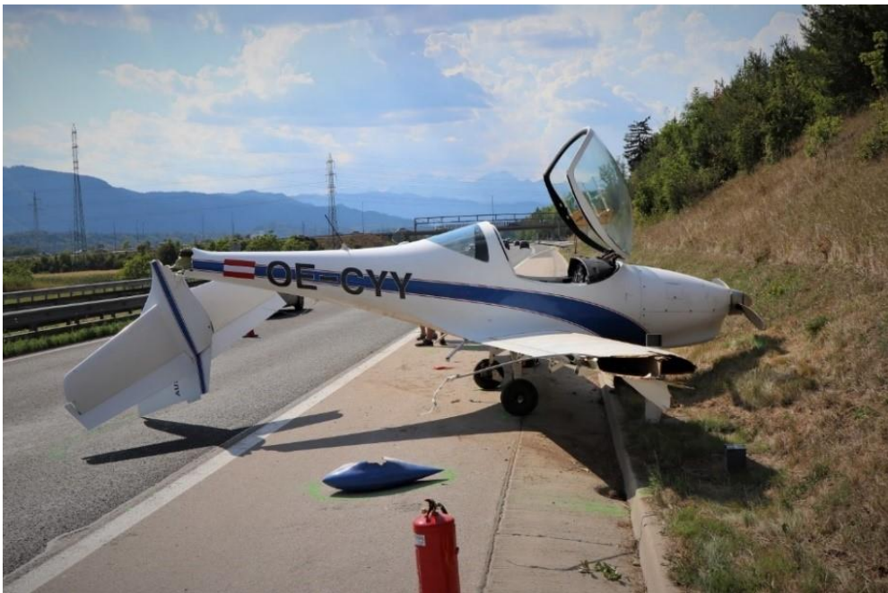
Figure 2: Position and damage of the OE-CYY at the stop point
