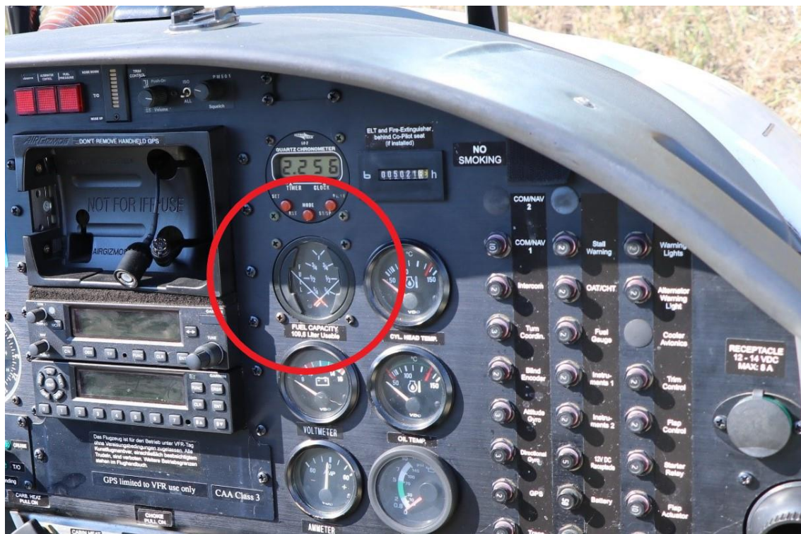
Figure 7: OE-CYY fuel gauge on the instrument panel in the aircraft cabin
