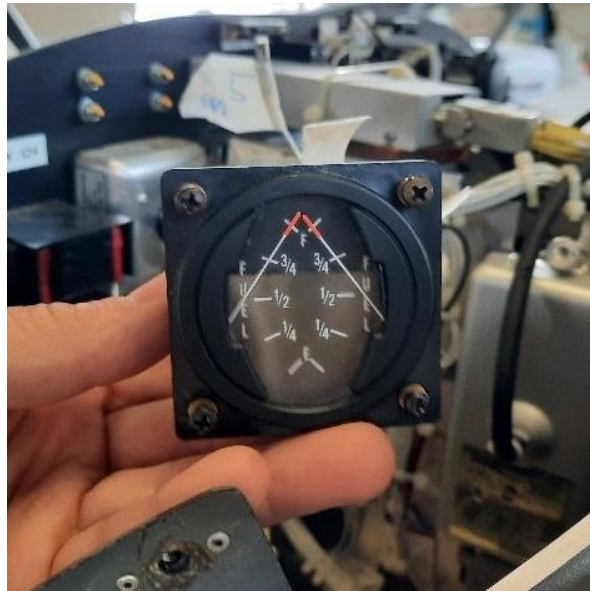
Figure 17: Indicators of the instrument when the GND contact is not connected
