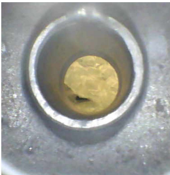
Fig. 5: GOOD Welding – the weld seam is uninterrupted around the pipes circumference.
